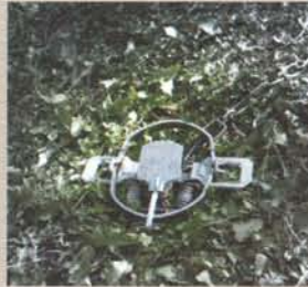
Double spring foothold trap in set position. The blades of metal on either side are what you step on to release it.
