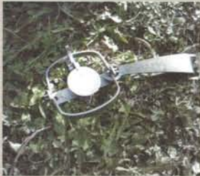
Single spring foothold trap in set position. Blade of metal to the right is the release.
