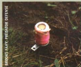
The upper two-inch portion of the M-44 is baited and exposed above ground.
